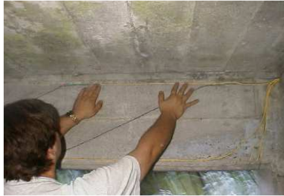
Fast Demodulation of Sensor T1FC (Transverse Beam, External to Composite, Flexure, Center) on Horsetail Falls Bridge, Demo
